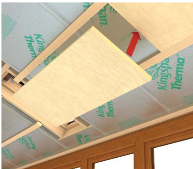
Install insulation between batten
